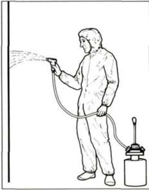
Use low-pressure spraying where possible
