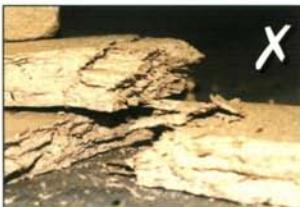
Broken asbestos insulating board, asbestos lagging and sprayed asbestos (limpet)
