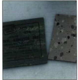
Floor tiles that contain asbestos can also have asbestos-paper backing, or be fixed with asbestos-containing mastic
