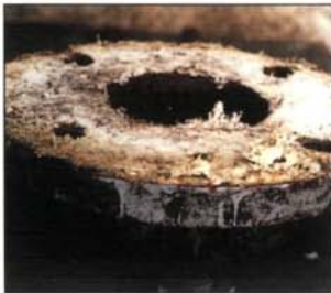
Gasket material left on a pipe flange
