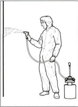
Use low pressure spraying
