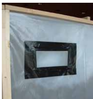
Figure 6.17 An enclosure being smoke tested
