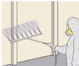
Figure 7.14 Multi-point spray system
