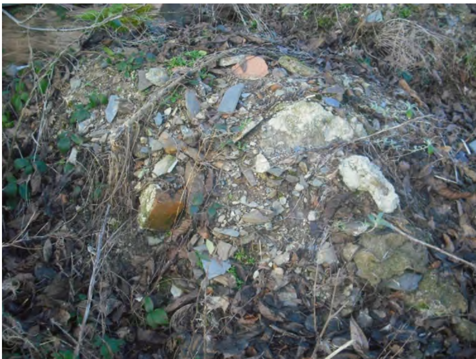
Figure A7.1 Fly-tipped material brought onto the site can be a source of asbestos
