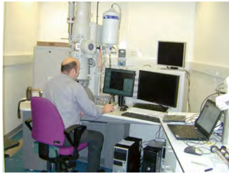
Figure A4.2 Transmission electron microscope in use
