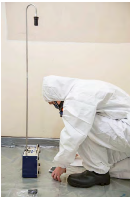
Figure 5.5 Analyst setting up a clearance test
