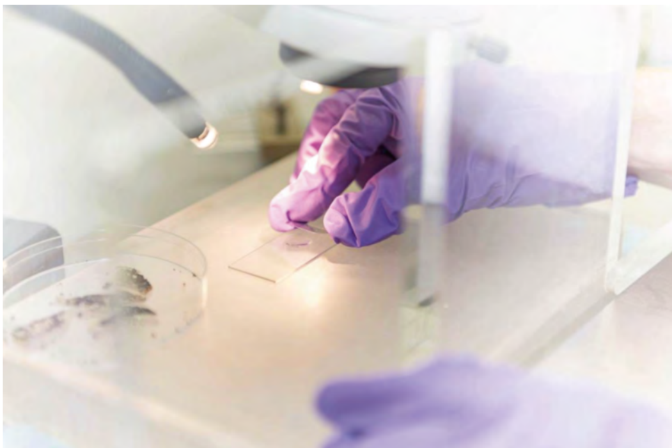
Figure A2.4 A glass slide with RI liquid ready for a fibre to be placed on it
