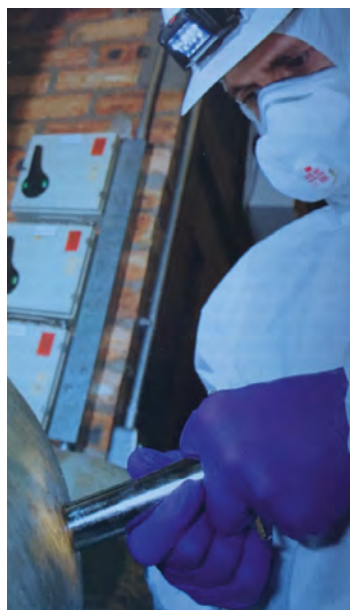
Figure 4.5 Analyst taking a core sample
