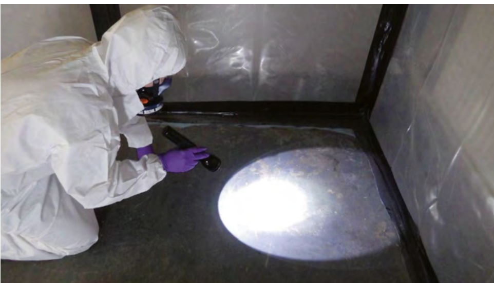
Figure 6.4 Analyst carrying out the thorough visual inspection
