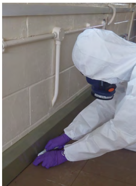
Figure 4.2 Sampling of a floor tile
