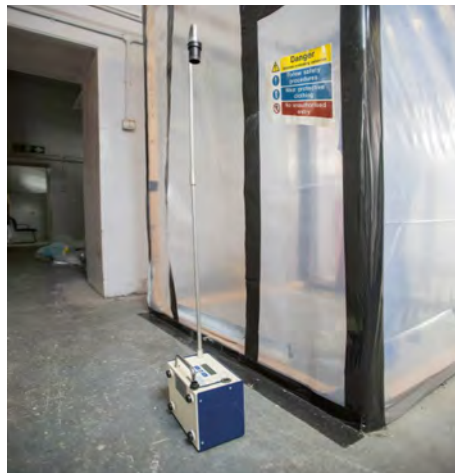
Figure 5.6 Leak test outside an airlock
