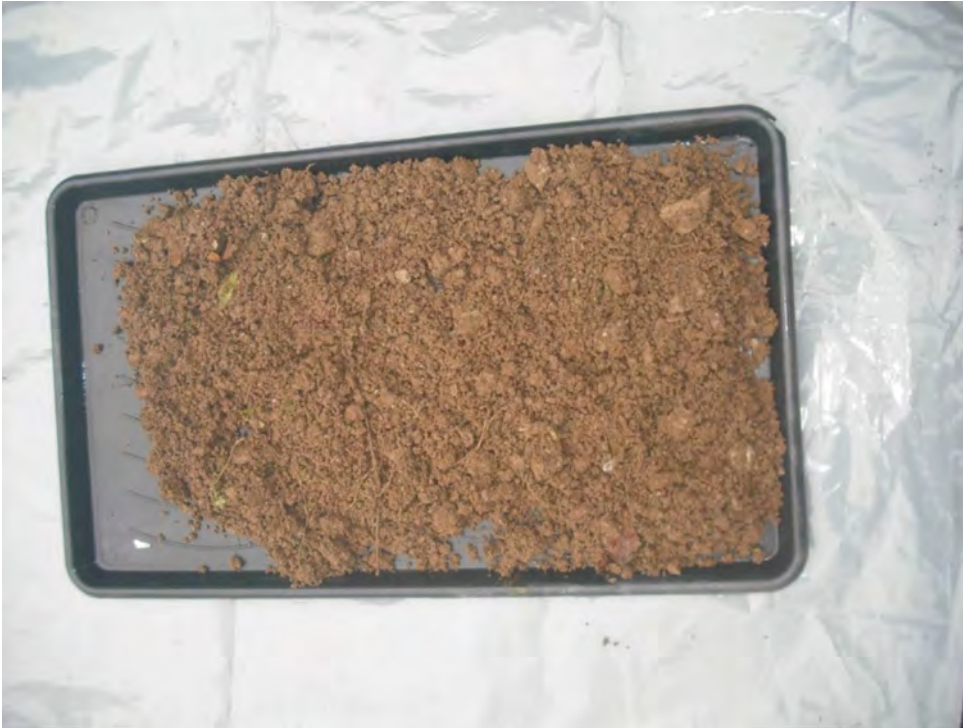
Figure A7.5 A 2-litre soil sample spread out on a 30 × 60 cm tray for visual inspection for possible fragments of asbestos
